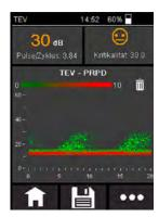
An indispensable function of the device is the phase pattern representation, so-called PRPD pattern. By means of this view, the user can clearly identify whether the measured data is due to partial discharges or simply noise – a big but decisive difference.
