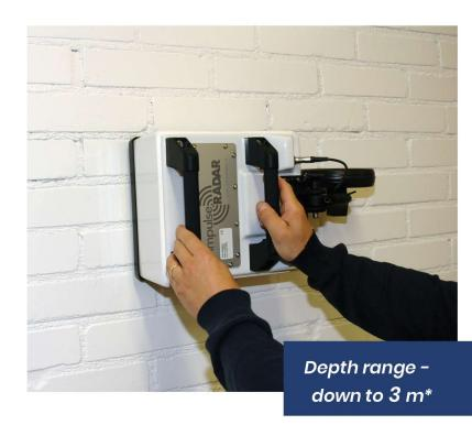
\*Figures for guidance only. GPR works best in high-resistive soils, absent of conductive layers. The actual depth range is dependent upon the di-electric properties of the ground or penetrable material under investigation.
