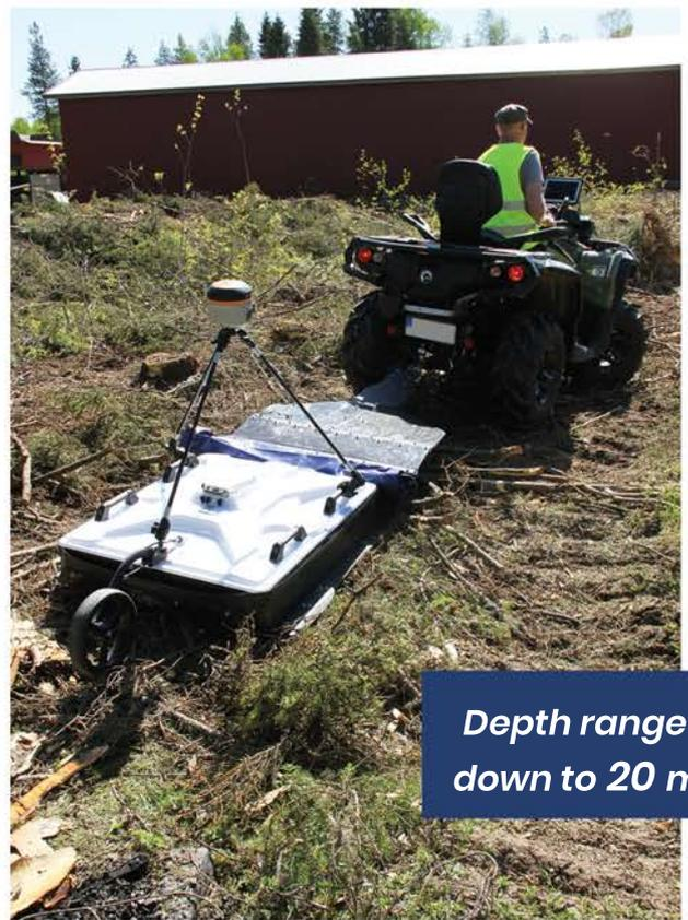
*\*Figures for guidance only, GPR works best in high-resistive soils, absent of conductive layers. The actual depth range is dependent upon the di-electric properties of the ground or penetrable material under investigation.*
