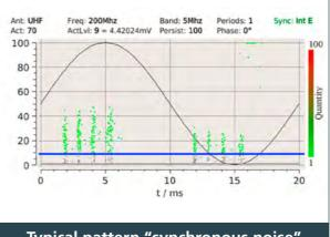
Typical pattern "synchronous noise" no PD - not critical
